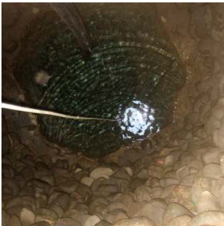
Slika 1. Meritev vodne gladine v gasilskem vodnjaku Latkova vas, dolina Bolske; julij 2011 (P. Souvent) Figure 1. Groundwater measurement in fire fountain in Latkova vas, Bolska valley; July 2011 (P. Souvent)
