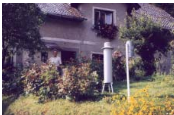
Slika 1.3.3. Opazovalec pred svojim domom, v ospredju stojita ombrometer in ombrograf, 16. 9. 1999 (foto: Filip Štucin) Figure 1.3.3. Observer's home and the rain gauge and recording rain gauge, on 16 th of Sept.1999 (photo: Filip Štucin)
